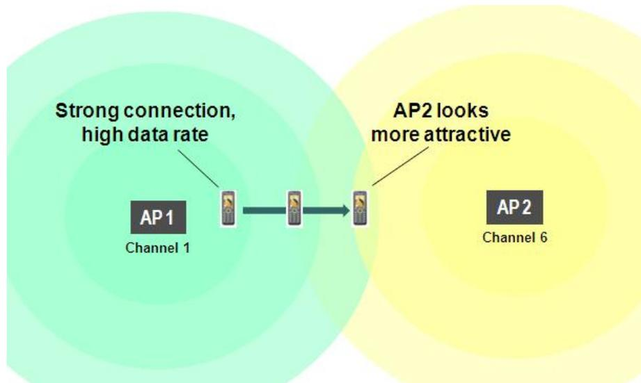
*As a client moves away from the AP to which it is associated, the client's connection becomes weaker, and the client may look for an AP that offers a better connection.*
