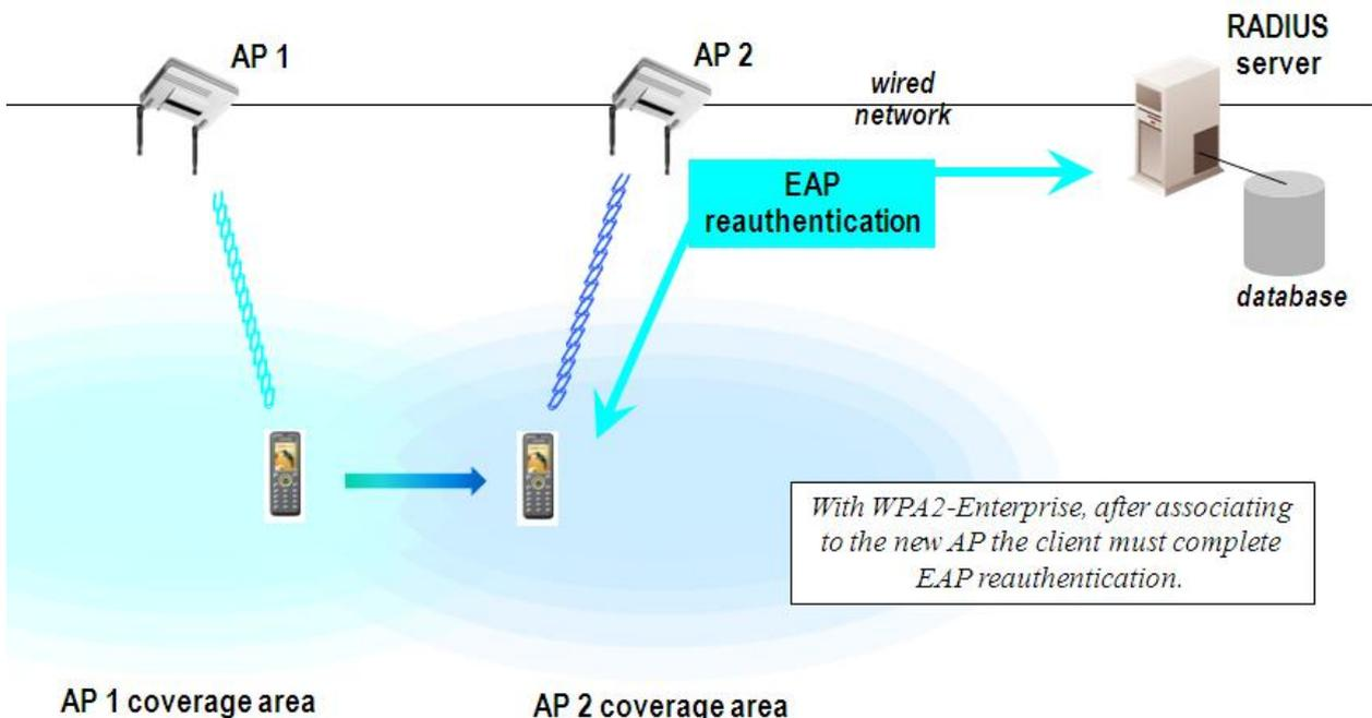
Standard EAP reauthentication requires interaction with an authentication server on the wired network.
